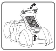
Locate the rectangular bar under the seat. Press the bar and lift the handle until the seat "clicks" in an upright position.
